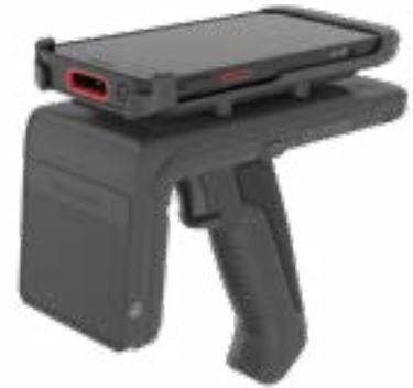
The Honeywell IH45 handheld RFID reader enables fast and accurate UHF RFID inventory capture for retail, transportation and logistics, and supply chain inventory application.
